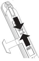
**6:** Remove Hook and Rotate to Proper Position
