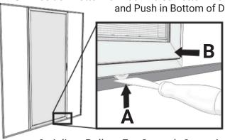
**9:** Adjust Rollers For Smooth Operation. Bottom Rollers Before Top Rollers
