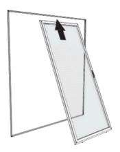
8: Position Bottom of Door. Raise Bottom Rollers (A) and Push in Bottom of Door (B)
